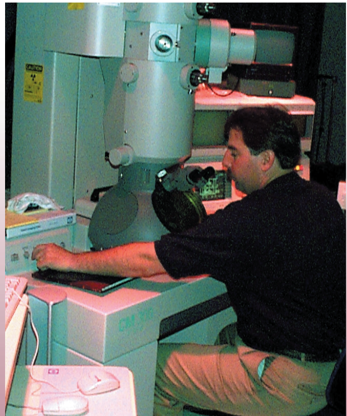
Microscopist Mark Wall uses the transmission electron microscope to image the microstructure of plutonium.
