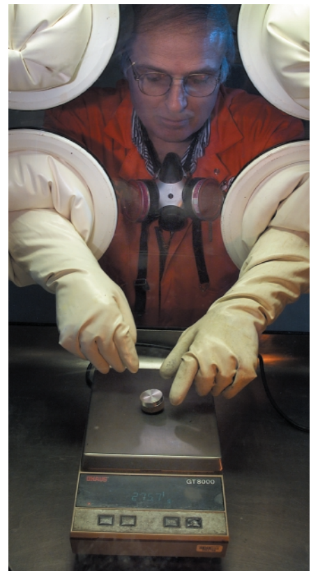
Machinist Bill Poulos, a trained fissile material handler, weighs a machined plutonium part in a glovebox in the Plutonium Facility's Radioactive Materials Area. He is using a certified balance that is part of the plutonium accountability system. Virtually all handling of plutonium is done in a glovebox such as this one.
