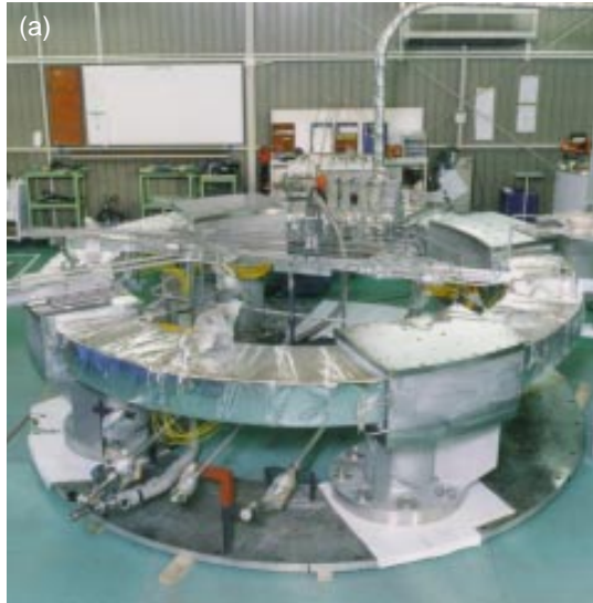
Figure 4. The Laboratory is testing (a) Toshiba Corporation's developmental superconducting coils at (b) Livermore's Superconducting Magnet Test Facility. Such magnet coils would be used as energy storage devices for emergency power.
