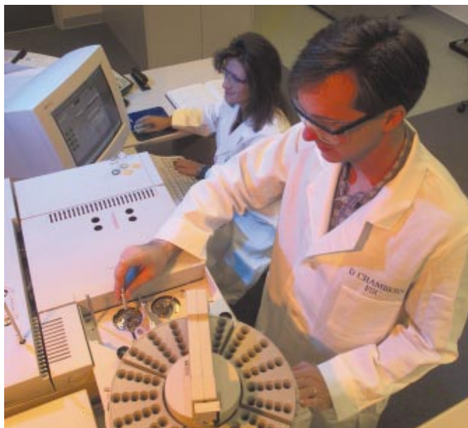
Figure 3. (above) Heather King and David Chambers demonstrate Livermore's solid-phase microextraction (SPME) sampling technique. The microfiber inside the syringe is coated with a special polymer that collects molecules of gas-phase chemicals. (right) The fiber is then desorbed in the injection port of a gas chromatograph-mass spectrometer, which identifies the compounds and measures their amounts.
