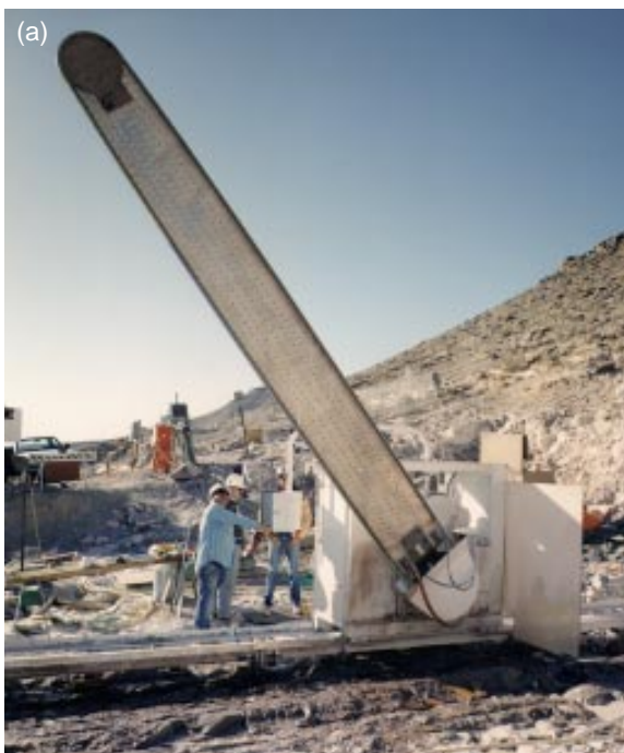
Figure 2. (a) Rock was cut out of Yucca Mountain in Nevada and (b) tested to determine hydrologic and geochemical characteristics.
