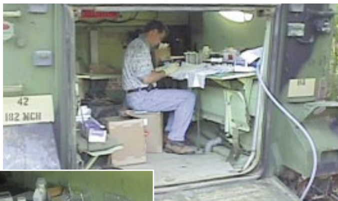
Figure 2. Livermore’s Jeff Haas sampled over 1,200 mortars in two days using the center’s unique thin-layer chromatography screening system.
