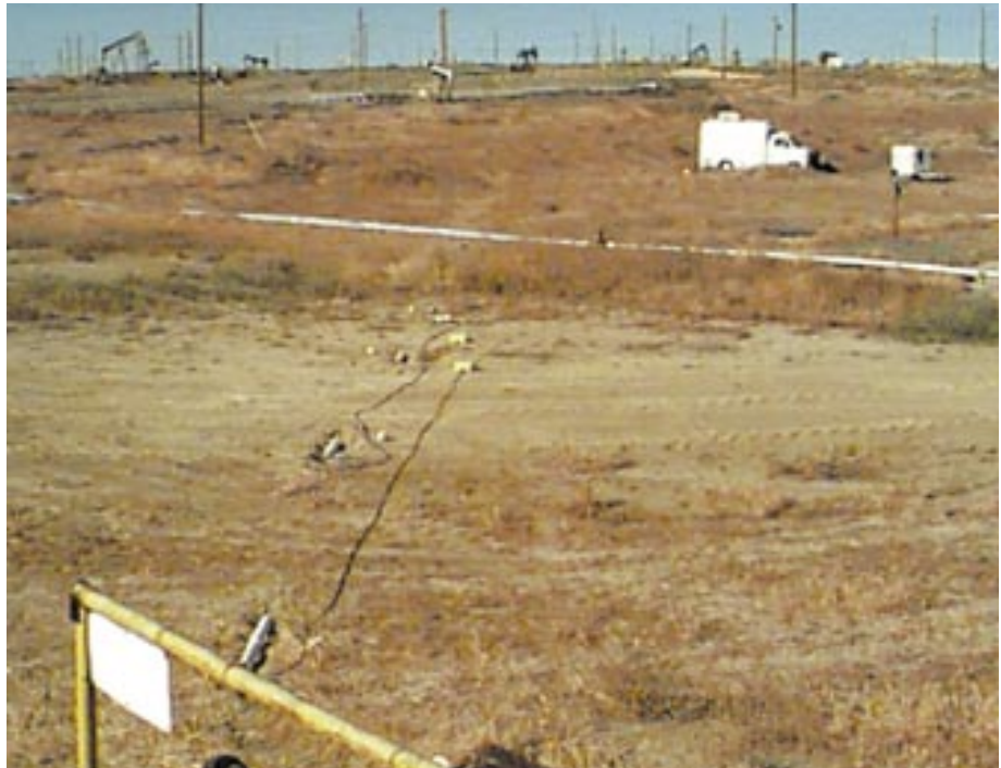
Figure 4. From the location of a magnetic field transmitter in a borehole at Lost Hills, California, radial magnetic field receivers can be seen on the surface at 5, 10, 15, and 20 meters along a survey line.
