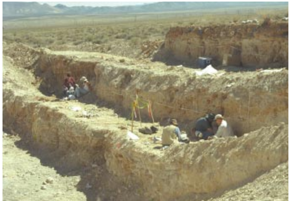
Figure 2. The trench at the Nevada Test Site for studying radionuclide movement in undisturbed soil is perpendicular to an earthquake fault. Two-inch cores were drilled horizontally about 24 inches deep. Samples were taken from six cores and from profiles, 15 to 30 feet apart. Two profiles are far from the cracked area, and the others are in the fracture area.
