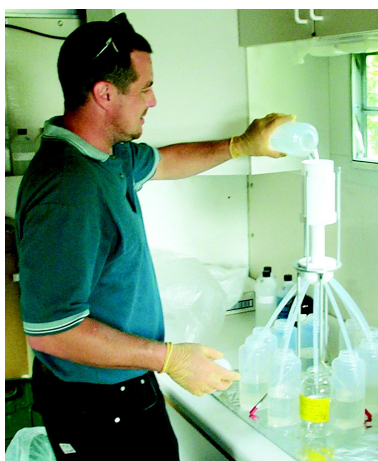
USGS personnel processing a water-quality sample using a Teflon cone splitter (photograph taken by J.B. Atkins, USGS).
