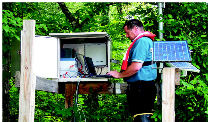
Programming data-collection platform for satellite telemetry of hydrologic data (photograph taken by J.B. Atkins, USGS).
