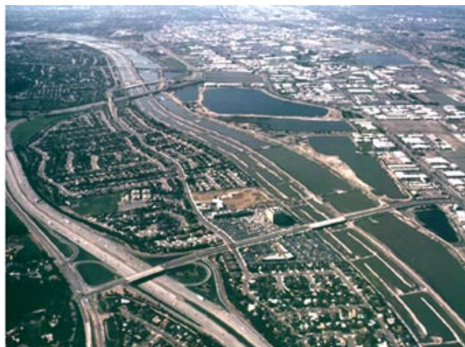
Figure 2. Orange County Water District uses abandoned gravel pits as spreading ponds to artificially recharge water to its aquifer.
