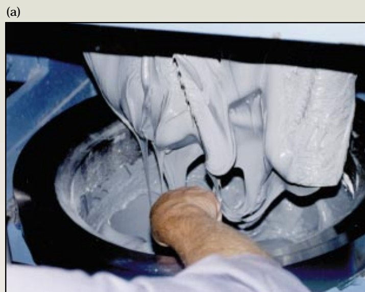
Figure 1. (a) This new explosive paste material was designed using CHEETAH to deliver high energy very quickly for use against armored tanks. (b) After formulation, it was used in an experimental shaped charge, which launches a copper metal jet in only 10 microseconds.
