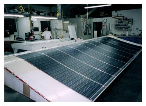
Figure 3. A wing section of Pathfinder in the shop after nine solar arrays were installed.
