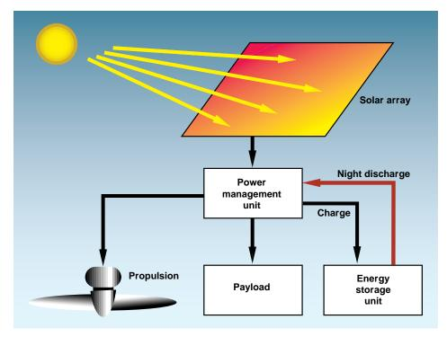
**Figure 1.** A simplified schematic of solar-rechargeable, round-the-clock flight. Less than half the sunlight striking the solar cells powers the motors; a larger fraction is stored on board. As the solar energy striking the cells falls below a certain minimum, the aircraftÕs powermanagement unit begins drawing on the stored energy for the ÒnightÓ portion of the flight.
