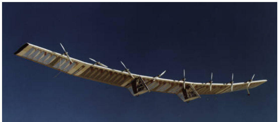
Figure 2. (a) Pathfinder on Rogers Dry Lake Bed before flight. The dark areas are the solar cells. Compare the slight droop of the wing with its position in (b), which shows Pathfinder in flight (altitude ~60 m). The upward curve of the wing results from lift, and this curvature of the wing puts its structural components in the condition of least load. However fragile Pathfinder might look, its flexibility and light weight allow it to withstand high wind gusts as it climbs to high altitude.
