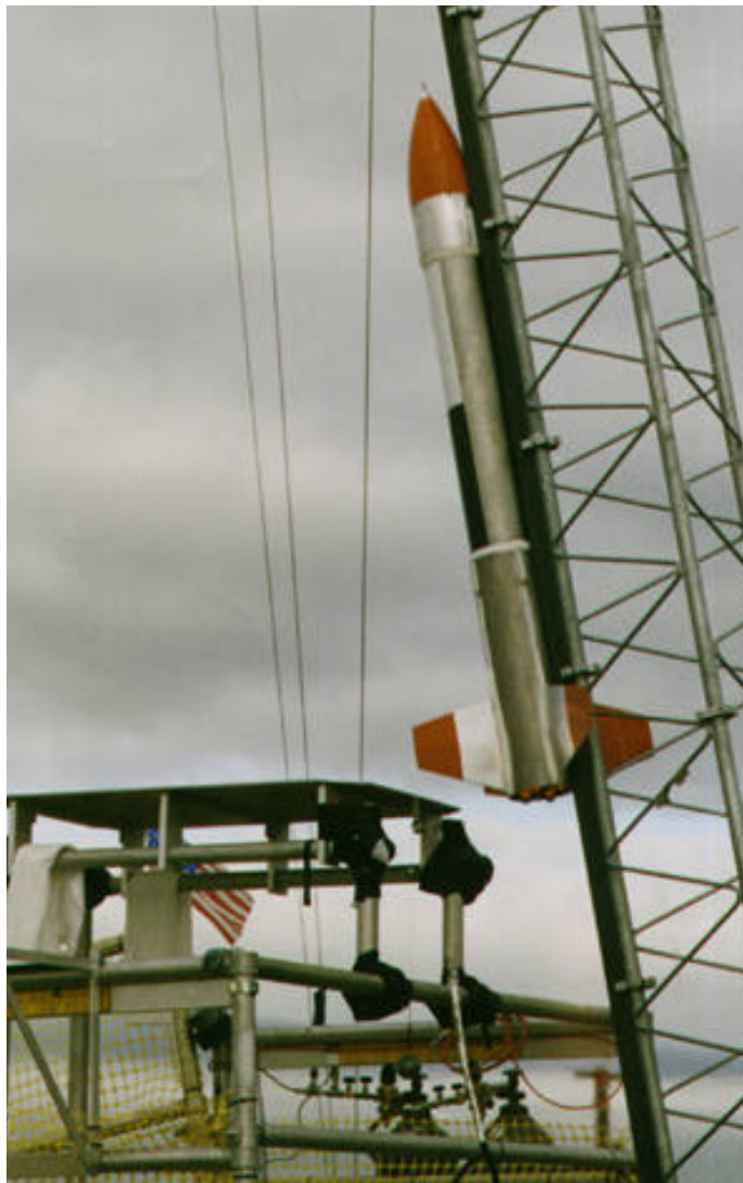
Figure 5. ASTRID ascends the launch rail on February 4, 1994. The glow of the four thrust chambers can be seen, but the plume is invisible because hydrazine fuel decomposes cleanly and at a lower temperature than other rocket propellants.
