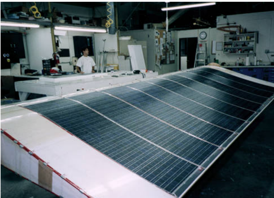
Figure 3. A wing section of Pathfinder in the shop after nine solar arrays were installed.
