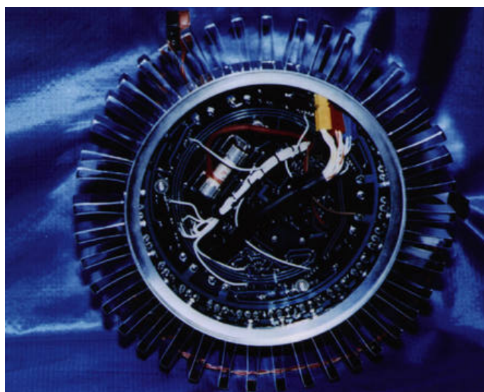
Figure 4. Two views of a Pathfinder motor: with propeller assembly (a) and without (b), showing its internal components and the radial cooling fins. There are only three moving parts in the entire assembly, as compared to more than 100 in the previous generation design.
