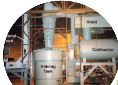
ERCo's innovative Vertical Flotation Melter Furnace
