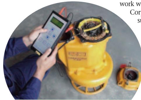
BJM technician performs a pump test
