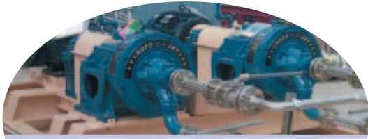
Roto-Jet pumps manufactured by Weir Specialty Pumps will be used for NOx suppression on gas turbine generators
