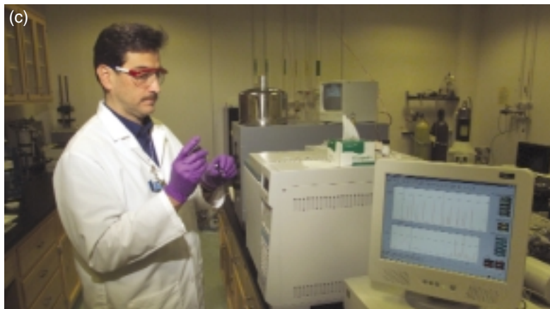
(a) Chemist Armando Alcaraz logs in a proficiency test sample. (b) Chemist Bob Maxwell holds a sample in a tube that will be placed in a nuclear magnetic resonance instrument (in background). (c) Alcaraz injects a microliter of sample into a gas chromatograph–infrared spectrometer system. (d) Chemist Hugh Gregg uses solid-phase extraction cartridges to clean a sample of hydrocarbon compounds that might mask a chemical warfare agent.
