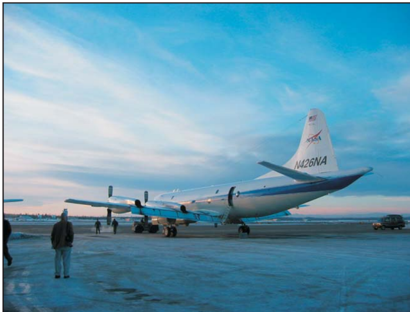
The NASA Wallops P-3B aircraft at Fairbanks International Airport. The P-3, equipped with high-resolution sensors, obtained validation data as part of the EOS Aqua AMSR-E Arctic sea ice validation campaign. The same platform has been used regularly to survey changes in Arctic land ice elevations.
