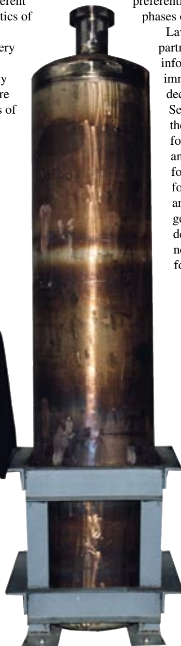
Leonard Gray, the chief scientist for Lawrence Livermore's Excess Fissile Materials Disposition Program, with a prototype stainless-steel canister, which is 3 meters (10 feet) tall and 60 centimeters (24 inches) in diameter and weighs 1,680 kilograms (about 2 tons).
