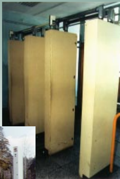
Figure 5. With the help of Livermore and other DOE laboratories, the Materials Protection, Control, and Accounting program has upgraded the safeguards and security at Russian weapons complexes. Shown here are (right) a pedestrian portal monitor and (below) a drive-through vehicle portal monitor.
