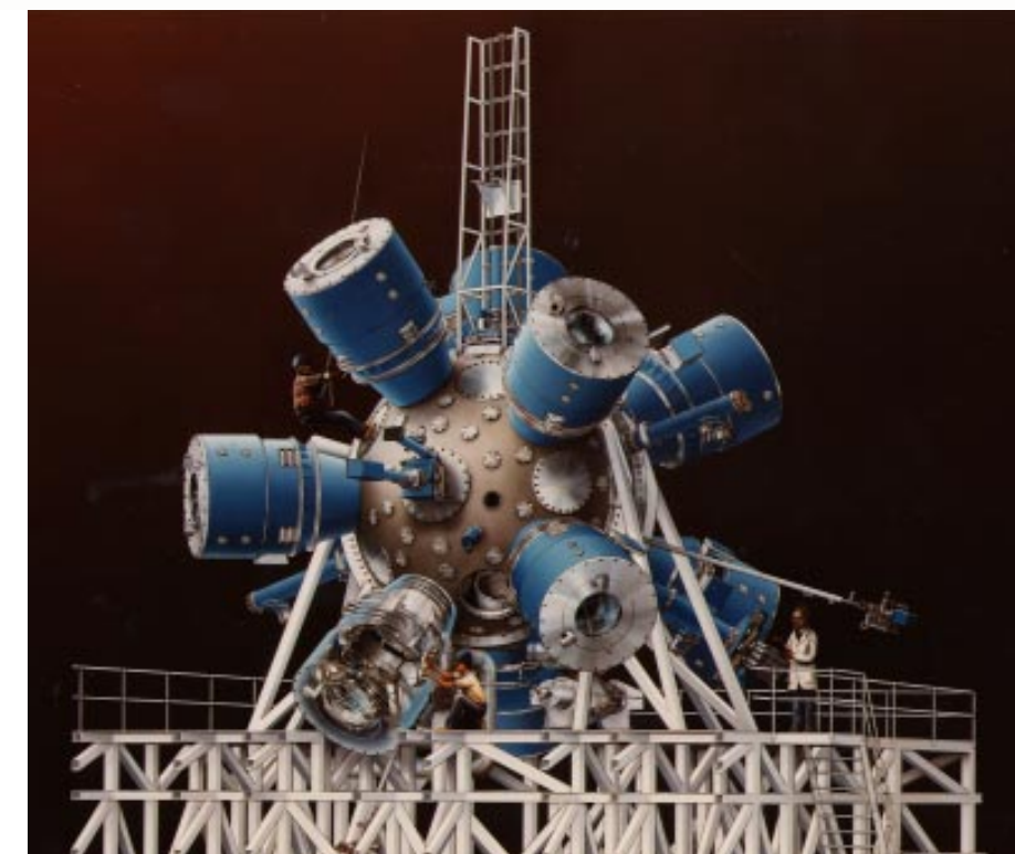
Figure 4. Artist’s rendering of the outside of the Nova target chamber, where the ten laser beams converge to heat and shock a tiny hohlraum. Note the two human figures at work on the platform. The entire structure is three stories high, and the spherical target chamber is 4.5 meters (15 feet) in diameter.
