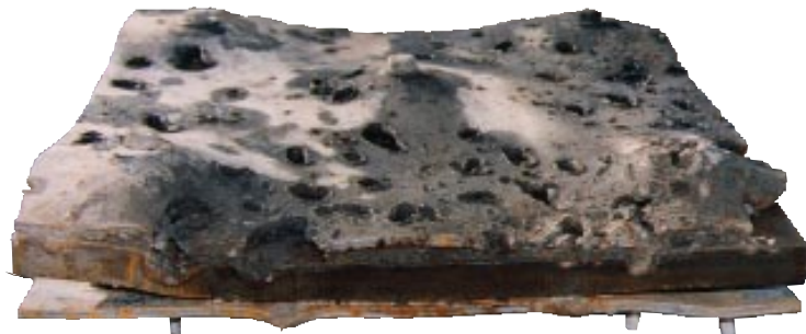
Figure 3. Shrapnel damage to a steel plate after a test to determine how much shielding is necessary for the firing chamber.
