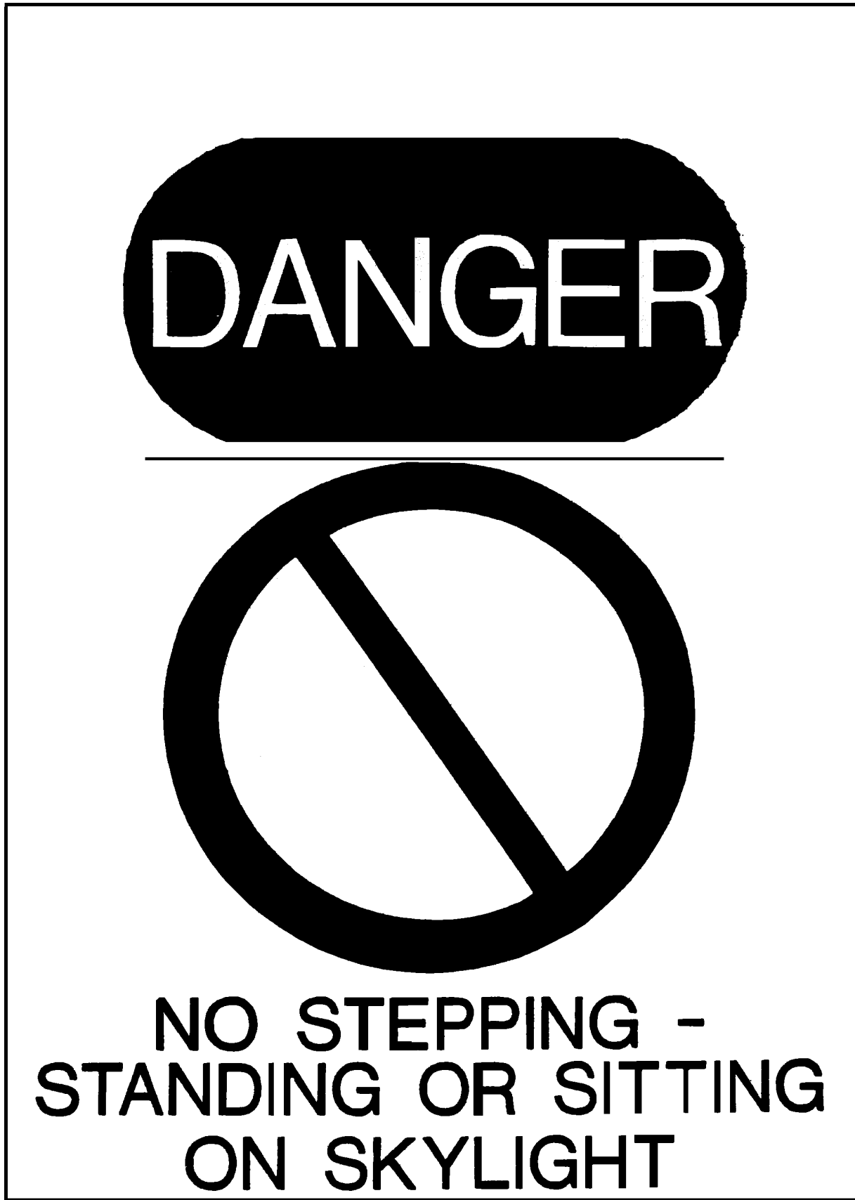
Figure 4. Recommended Accident Prevention Sign to be Applied to Skylights.
