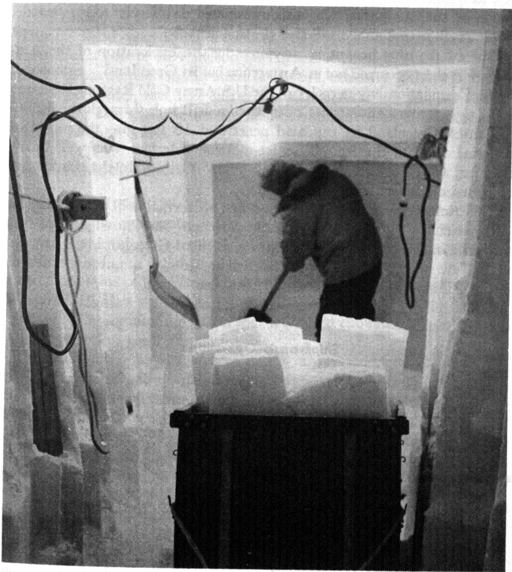
Figure 10.—Samples from this deep snow pit at Byrd Station, Antarctica, are being analyzed to determine the concentration of common lead precipitated from the atmosphere during the last 60 years.
