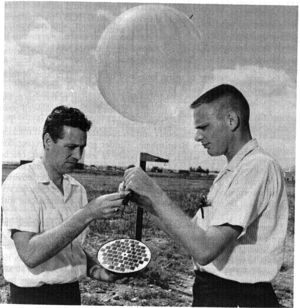
Figure 4.—Scientists prepare to attach solar-powered transmitter to GHOST balloon to be launched from Christchurch, New Zealand. The 6-foot balloons, designed to float at fixed altitudes up to 40,000 feet, are providing the first direct information on the flow of air around the world in the Southern Hemisphere.
