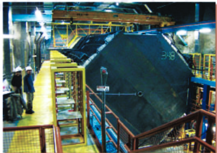
The MINOS detector with 348 of its 450 detector planes in place.
