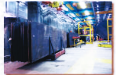
A dozen steel plates ready for assembly.
