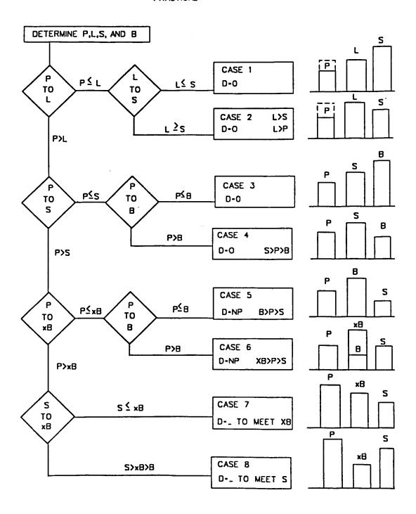
Figure 1. Possible conditions for comparisons of runoff concentrations with sediments
