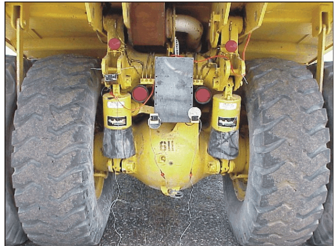
Figure 38.—Rear Guard sensors mounted on rear of dump truck.
