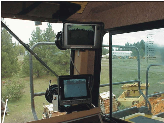
Figure 7.—Two types of monitors mounted in cab of dump truck.
