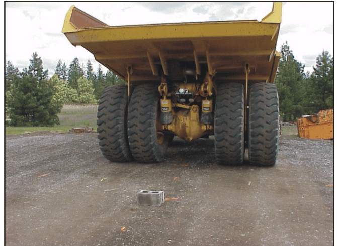
Figure 5.—Detecting a cinder block.
