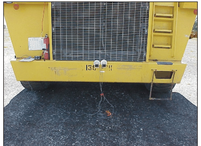
Figure 42.—Rear Guard system's ultrasonic sensors mounted close together on front bumper.
