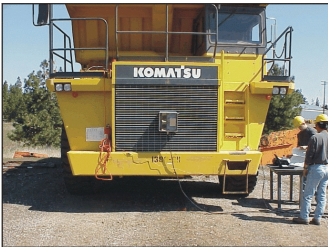
Figure 29.—Ultrawide-band radar system mounted on front grill.
