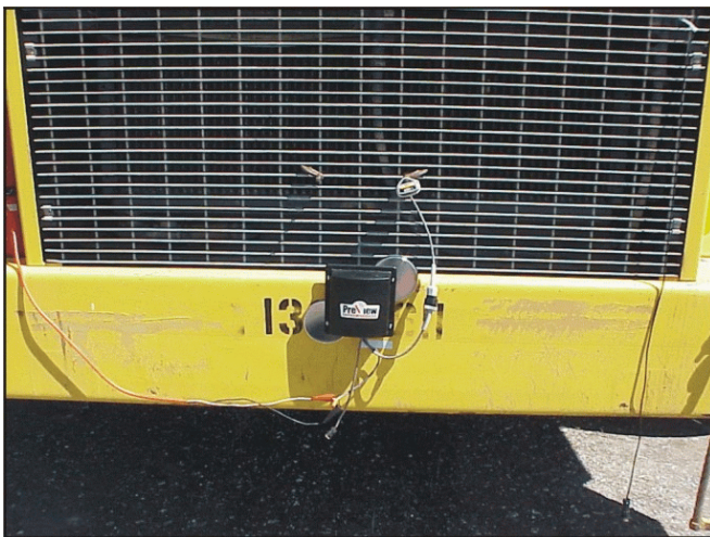
Figure 22.—Preview radar system mounted on front bumper.
