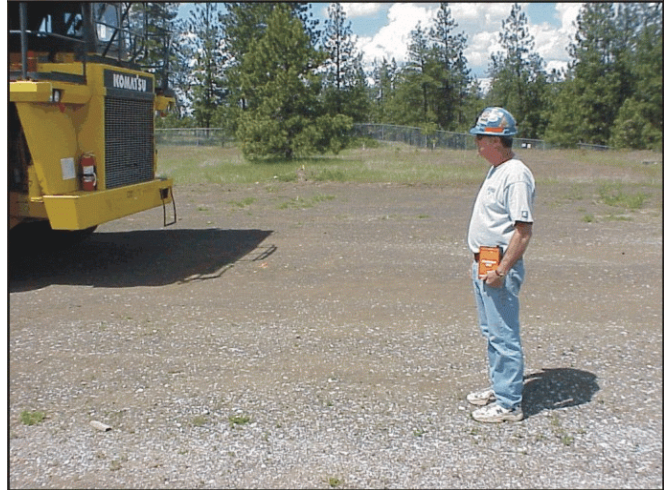
Figure 36.—Determining detection zone of Buddy system and a person.
