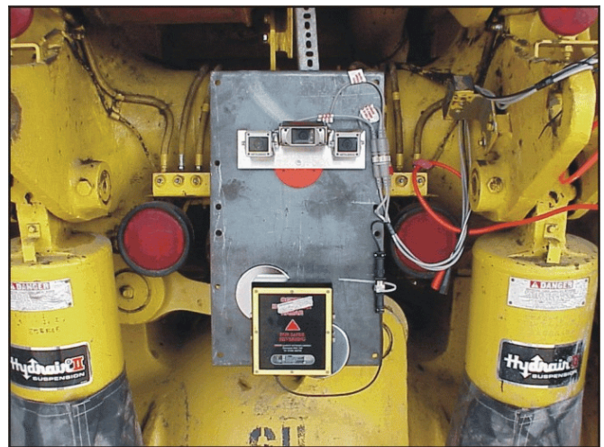
Figure 6.—Sensor Vision system mounted on rear of dump truck. Cameras are on top and radar unit is on the bottom.
