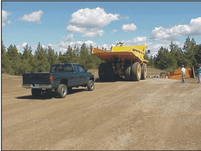
Figure 4.—Determining detection zone for a pickup truck.
