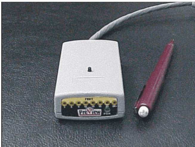
Figure 19.—Preview radar system display.
