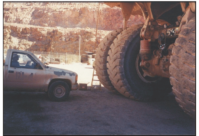
Figure 45.—Determining detection zone for a pickup Caterpillar 793B.
