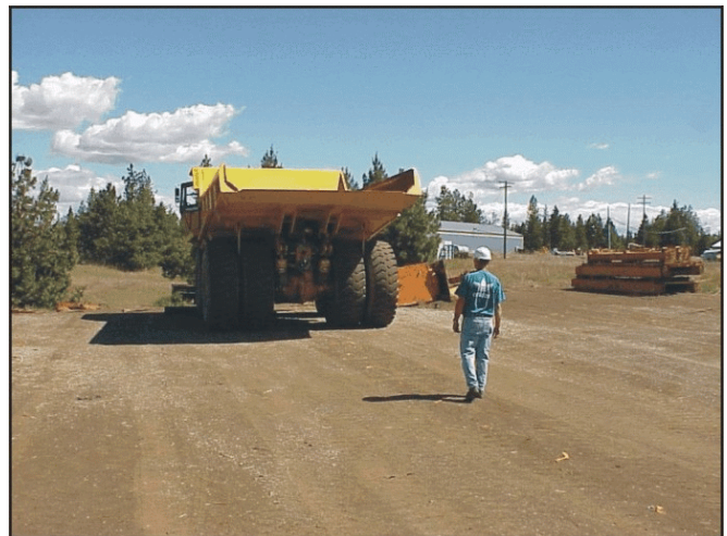
Figure 3.—Determining detection zone for a person.
