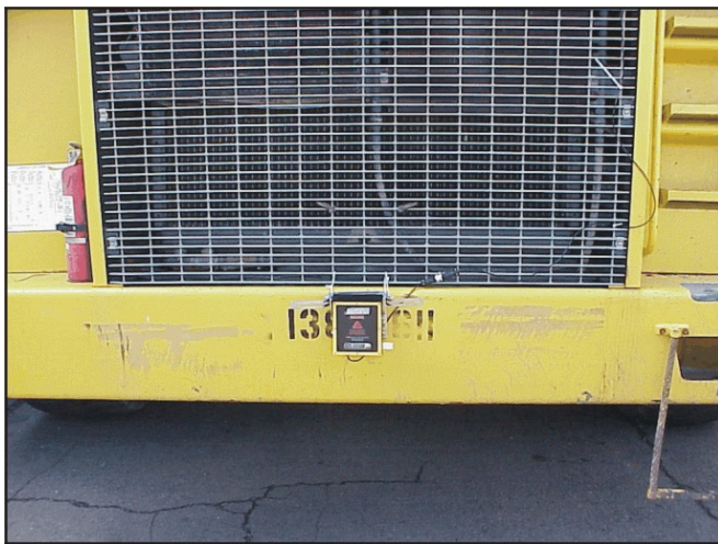
Figure 11.—Ogden radar system mounted on front bumper.
