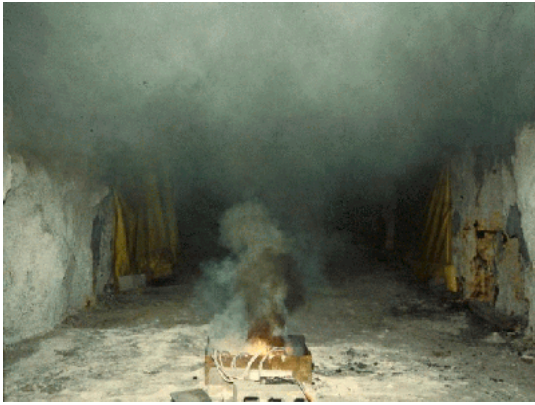
Coal fire detection experiment in the Safety Research Coal Mine.
