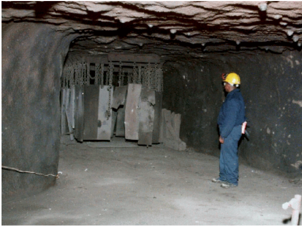
Chamber in the mine where toxic fume measurements are conducted. The steel plates protect the chamber from shrapnel produced by the detonation of the pipe bomb.
