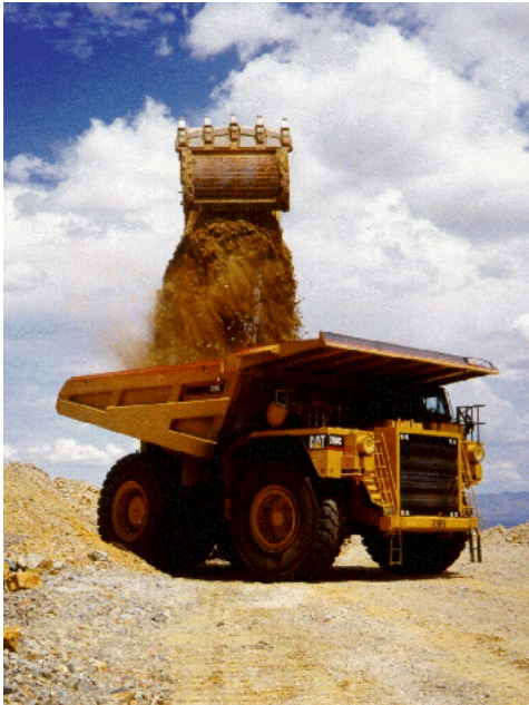
Dropping load into haulage truck creates impact shock for the truck operator.
