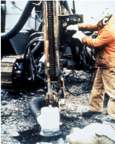
The operation of mining equipment, (e.g., the drilling of rock) can contribute to high noise levels.
