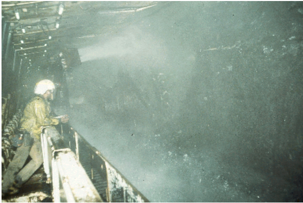
Dust generation and water spray application at an operating longwall face.
