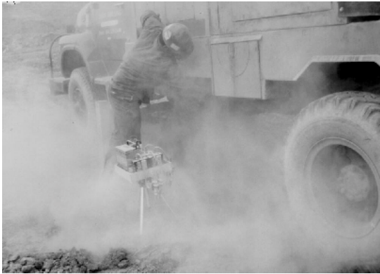
Dust sampling array for assessment of respirable dust concentrations.
