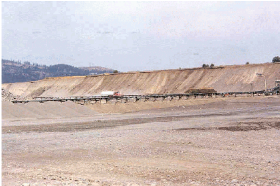
Transport of talc by tramlines generates dust.
