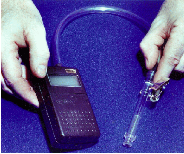
The dust dosimeter has two components: a small pump and a dust detector tube.
