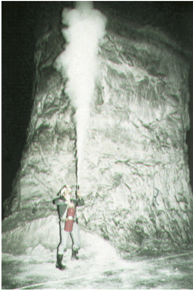
Vertical exhaust trajectory from a fire extinguisher is unaffected by the underground mine ventilation air flow.
