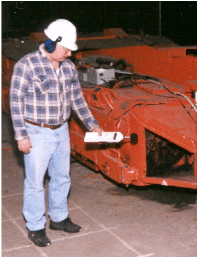
Noise measurements being made on a continuous mining machine.
