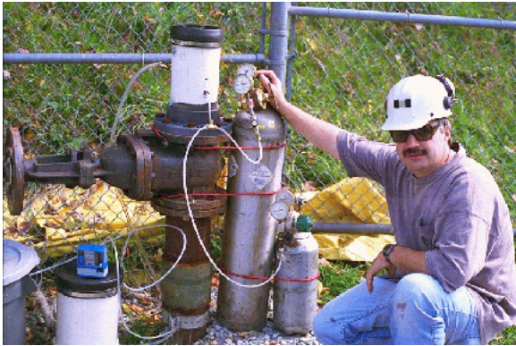
A NIOSH researcher prepares to inject sulfur hexafluoride tracer gas into a gob gas venthole to determine gas flow paths in the longwall gob.
