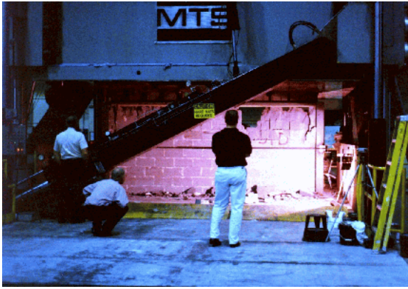
Failure of a mine ventilation stopping in the mine roof simulator.
