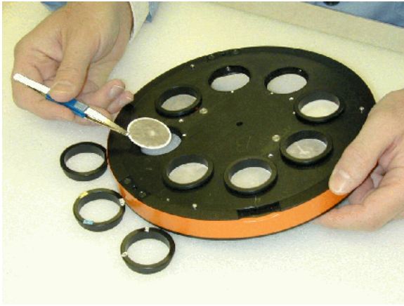
An eight-filter sample wheel speeds analysis by automated sample handling and alignment.
