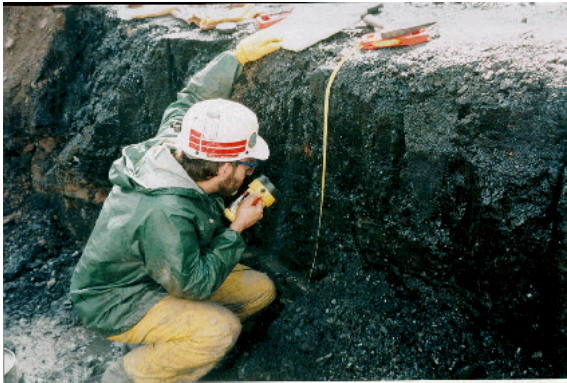
Field description of coal compositional banding in the Lower Kittanning Coalbed prior to collecting a channel sample at a surface coal mine.
