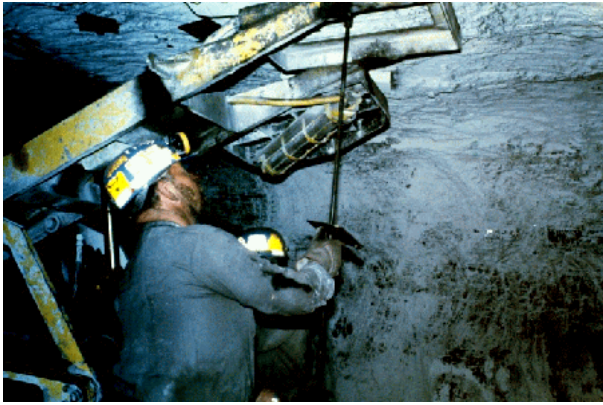
Field assessments are measuring the roof bolter operator's exposure to respirable silica dust.
