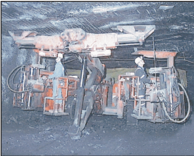
Figure 12.—Walk-through chassis roof bolting machine. (Photo courtesy of J. H. Fletcher and Co.)
