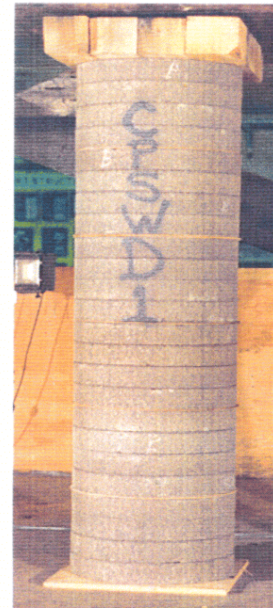
Figure 22.—The stiffness of a concrete crib is reduced by placing wood timbers on top.
