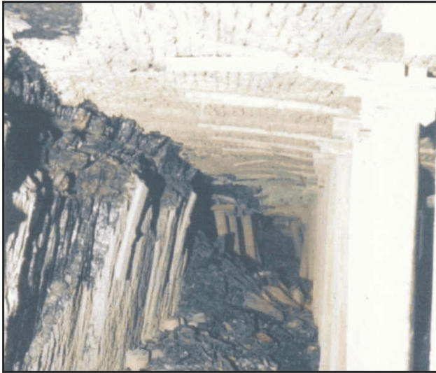
Figure 12c.—First open crosscut intersection inby the face supported with Propsetter supports.
