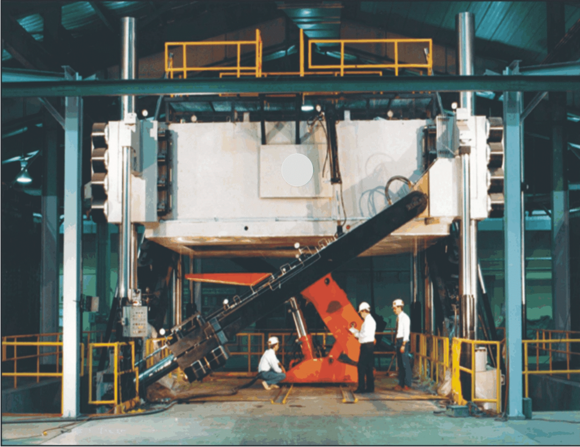
Figure 1.—The Mine Roof Simulator at NIOSH's Pittsburgh Research Laboratory.
