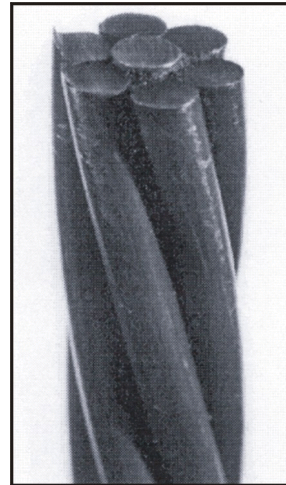
Figure 1.—Seven strand steel cable used to make cable bolts.
