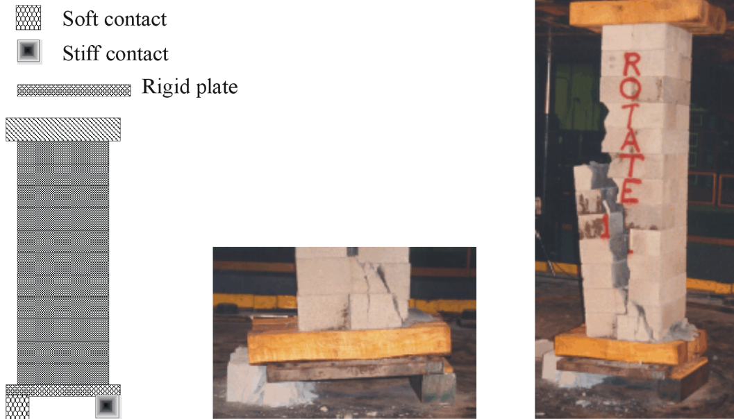
Figure 4 - Floor heave simulation and examples of support testing.
