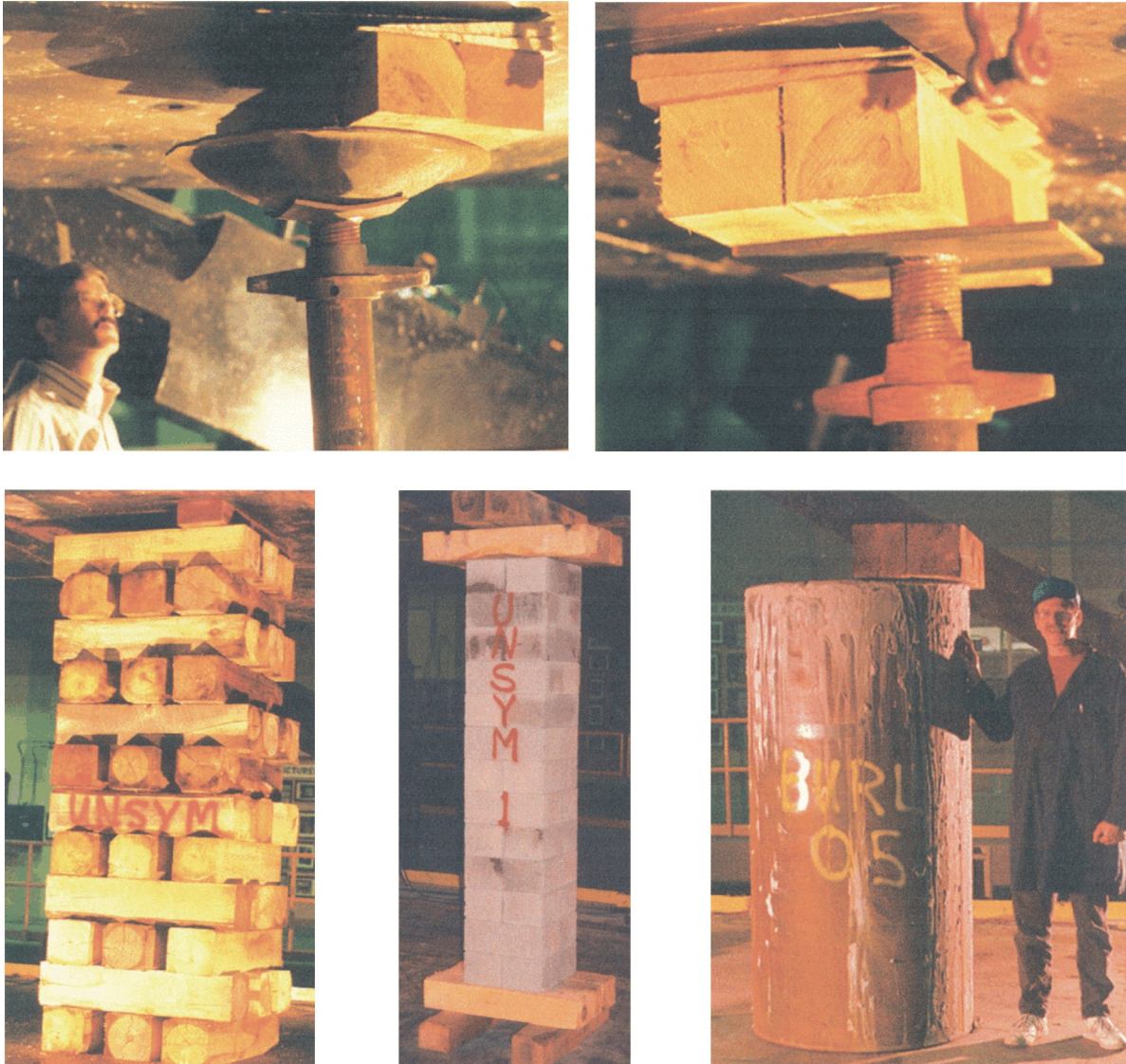
Figure 3.—Examples of asymmetric loading conditions.
