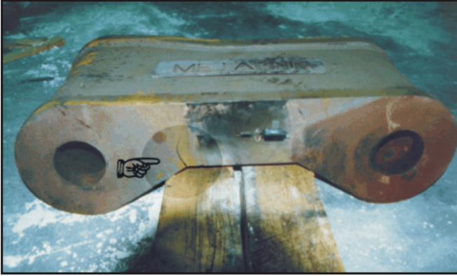
Figure 13.—Failure of bottom lemniscate link.
