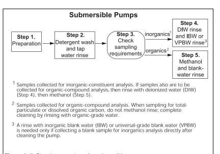
**Figure 3–5.** Cleaning procedures for submersible pumps.
