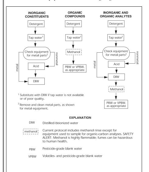
**Figure 3–1.** General sequence for cleaning equipment before sampling for inorganic and (or) organic analytes.
