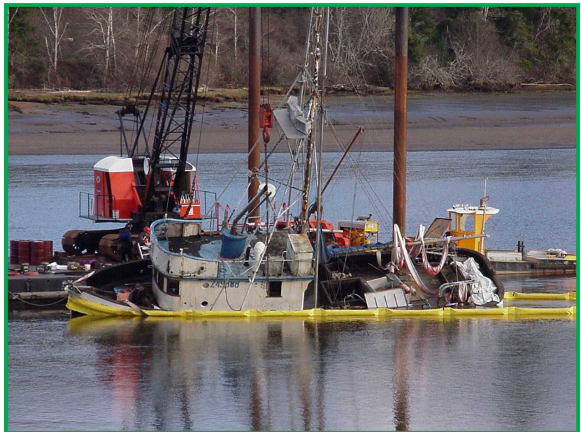
A barge with a crane lifts the sunken and leaking West Wind out of the water and hauled her back to port for repairs.
