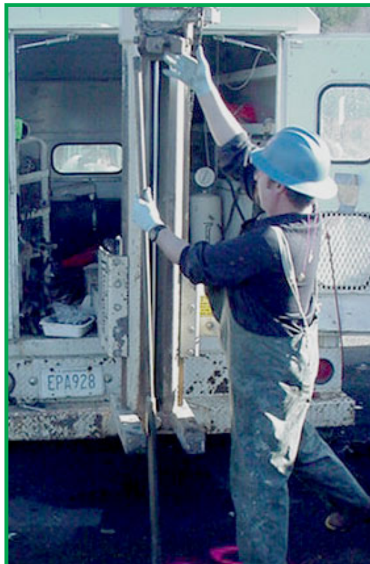
A worker at STEDCO Mill drills soil samples.
