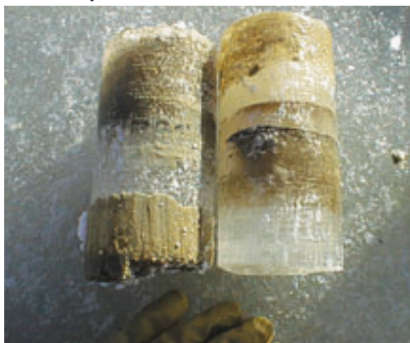
Figure 15. Photographs of samples collected for measuring ice-crushing strength at ice-data collection sites in South Dakota.
