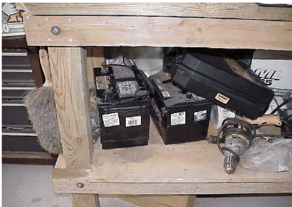
Improper Battery Storage
