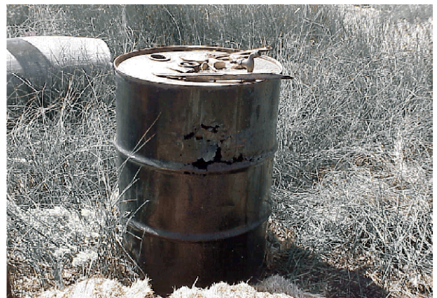
55-Gallon Drum of Unknown Liquid - Rusted Through at Top
