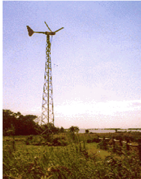
Bergey Excel 10kW Wind Turbine at Eastern Neck NWR
