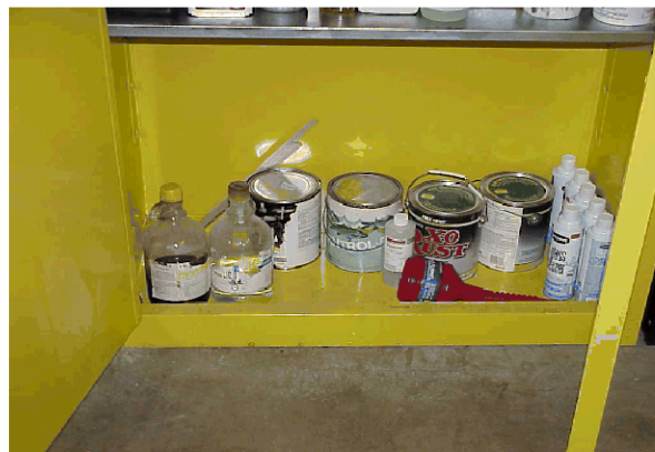
Incompatible Storage - Acids with Flammables
