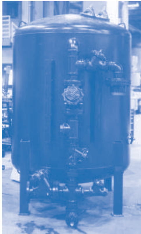
Figure 7-7. Pressurized Media Filter (USFilter).
