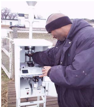
Scott Williams, technician for the Northern Cheyenne Tribe's Air Quality Program, changes a filter on a PM monitor.
