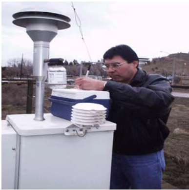
Jay Littlewolf, Administrator of the Northern Cheyenne Tribe's Air Quality Program, checks PM monitoring equipment.
