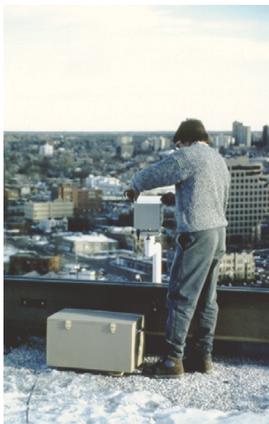
Testing visibility with an IMPROVE monitor. 17
