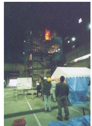
A flame extended from the third floor level was ejected from the open door on the 4 th floor.
