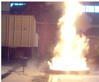
2.4 m diameter gasoline fire with 7 m tall flame at the time of CAF activation.
