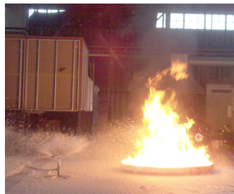
Gasoline fire at 15 s after CAF activation (2.5 m flame height).
