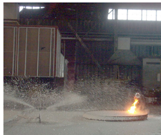
Gasoline fire at 30 s after CAF activation (fire controlled).
