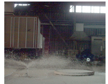
Gasoline fire at 45 s after CAF activation (fire extinguished).
