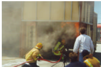
University of Canterbury measures CAFS performance for structural fire fighting.
