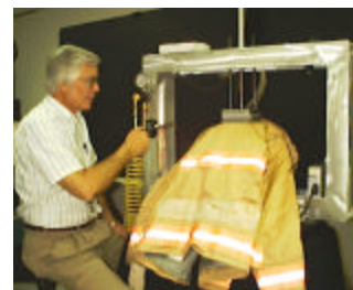
Ned Keltner of Ktech Corporation measures thermal protective properties of protective clothing.
