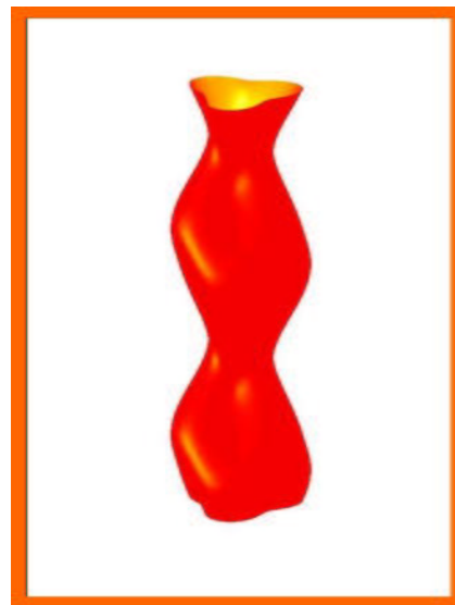
Shape instability of a quantum wire with a surface tension anisotropy having a three-fold axis of symmetry with respect to the wire centerline.
