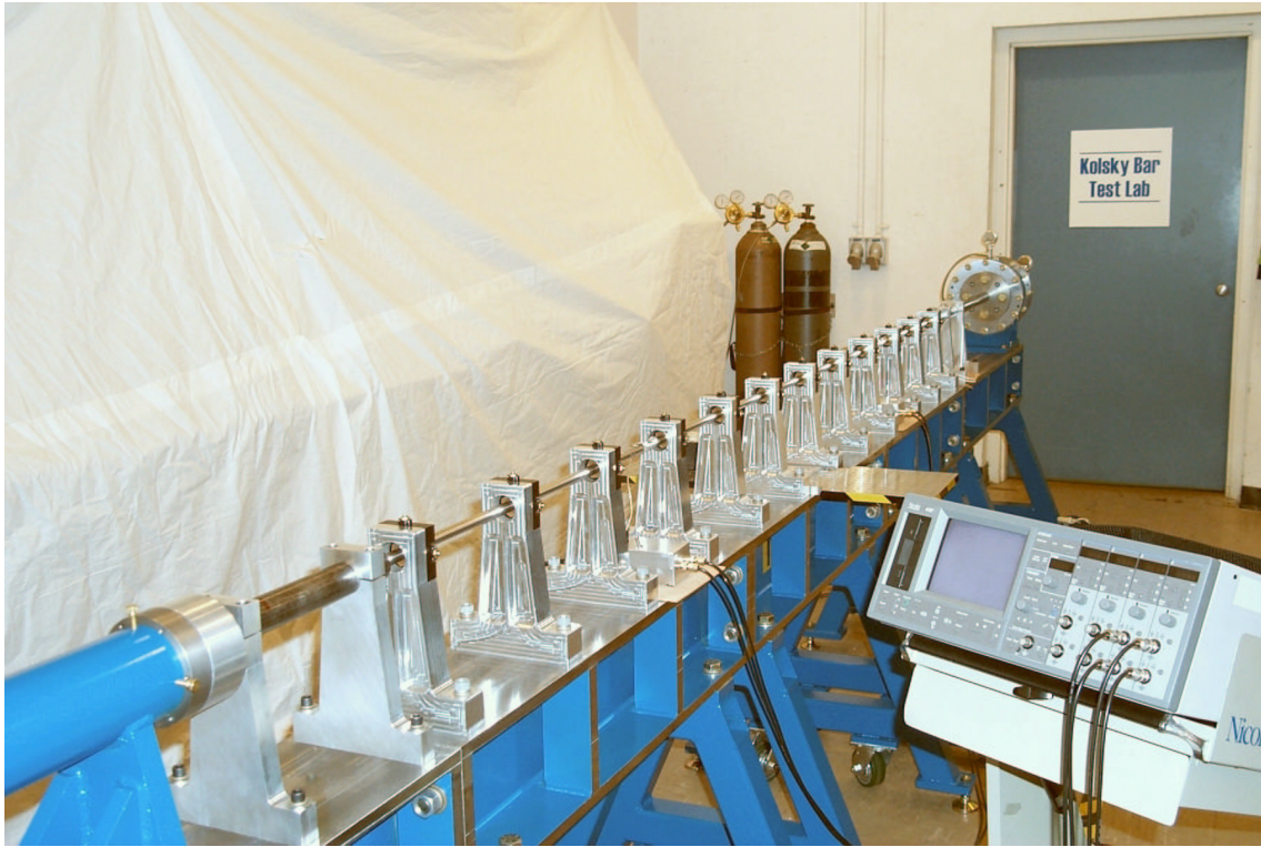
The NIST Kolsky Bar Facility in the Special Projects Building, showing the gas gun, bars, momentum trap, and data acquisition system.
