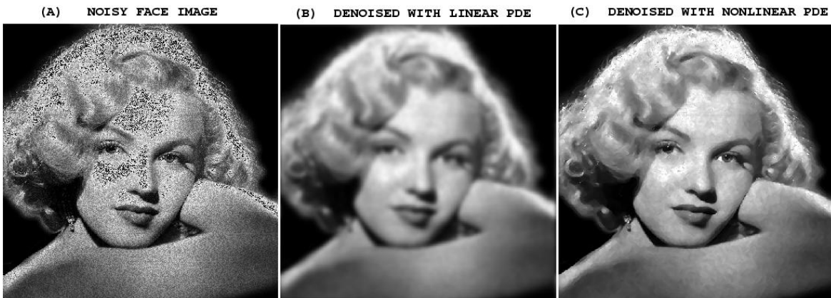
Figure 1. Advantages of nonlinear PDE approach in denoising. (A) Noisy Marilyn Monroe image. (B) Denoising with linear isotropic heat equation blurs the image. (C) Denoising with nonlinear anisotropic diffusion equation preserves life like features.
