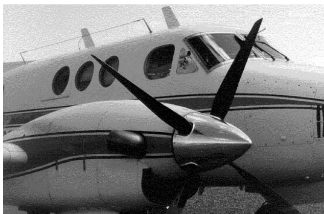
Figure 2. USDA Forest Service Air King 90. The smoke intake is visible in the side cockpit window. The pilot sat on the other side of the cockpit.
