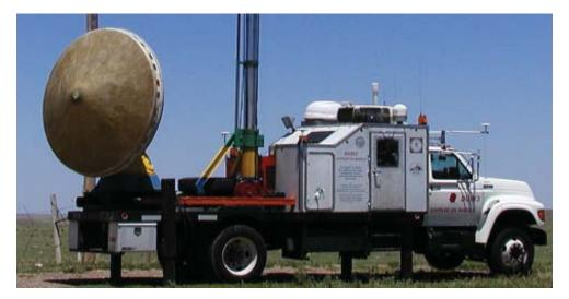
The Doppler on Wheels Project has created three mobile Doppler weather radars mounted on trucks that have explored rare, short-lived and small-scale phenomena, permitting the first-ever mappings of tornado winds, hurricane wind streaks, and resolution of detailed tornado structure and evolution at scales well below 100 meters. CREDIT: Ling Chan, Doppler on Wheels Project, Center for Severe Weather Research
