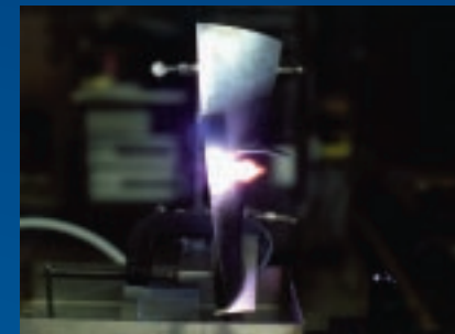
Laser shot peening— With Metal Improvement Co., Inc., we are developing a shock-peening tool for inducing deep compressive stress in metal surfaces (jet-engine fan blade shown)
