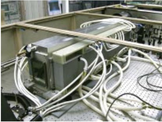
A heat capacity laser testbed using flashlamps as a surrogate pump source operated to investigate beam quality limits. A 100-kW diode-pumped prototype is being developed for the Army's High Energy Laser Strategic Test Facility.
