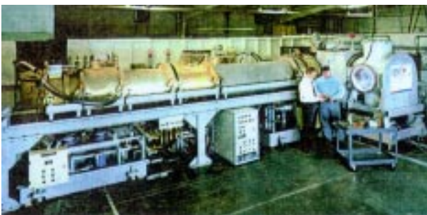
Repetitive pulsed power drivers for commercial ion beam surface treatment at SNL.
