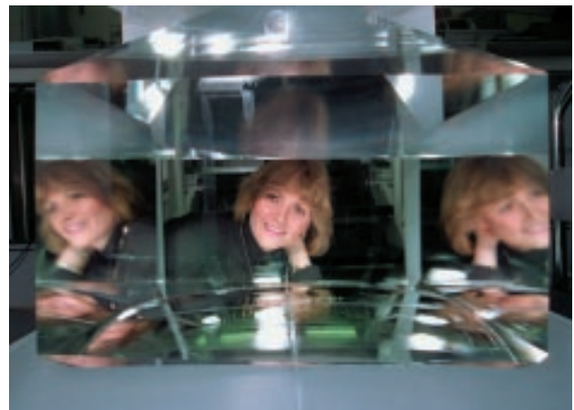
Potassium dihydrogen phosphate (KDP) crystal created with rapid-growth method.
