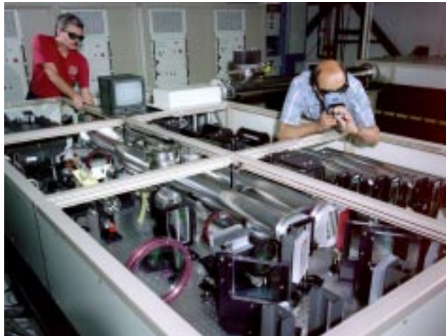
A zig-zag slab Nd:glass laser producing 60-J green output at <2\times diffraction limited at 3 Hz for Advanced Imaging Testbed experiments by the Air Force. This technology is also used for laser peening.
