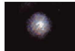
Nearly diffraction-limited focal spot shows focus quality of the foldable lens.
