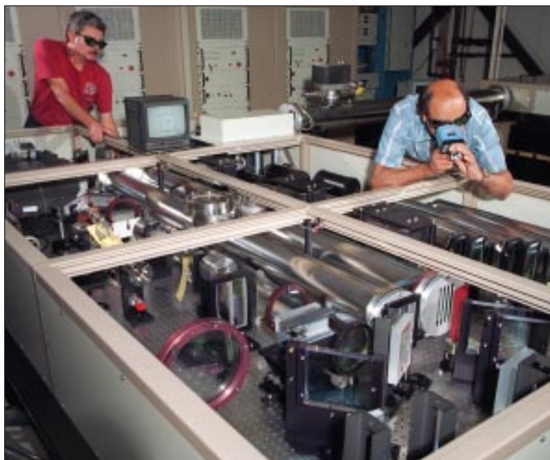
A flashlamp-pumped Nd:glass zig-zag laser (60-J, 600-ns green pulses at 3 Hz with 2 \times diffraction-limited beam quality) for the Air Force's Advanced Imaging Testbed project at the Starfire Optical Range for use as a satellite illuminator.
