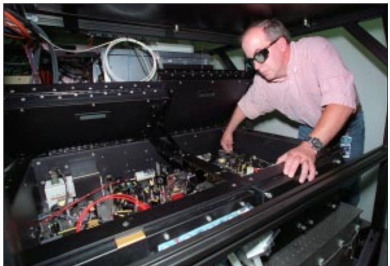
A compact, high-repetition-rate, frequency-agile, solid-state DIAL system (3 W at 10 kHz, tunable 3–4 \mu\text{m} , optical parameter oscillator) for airborne chemical sensing experiments.
