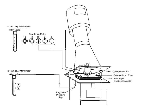
Figure 12. Calibration of a typical volumetric flow controller (VFC).
