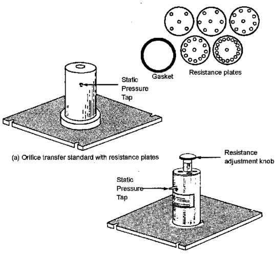
(b) Variable resistance orifice transfer standard
