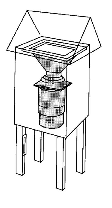
Figure 1. High-volume sampler with shelter.
