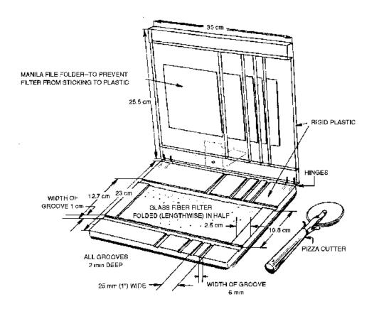
Figure 1. Example of templates for cutting filters.
