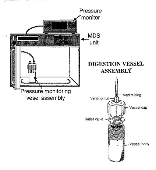
Figure 3. Example of microwave digestion system.
