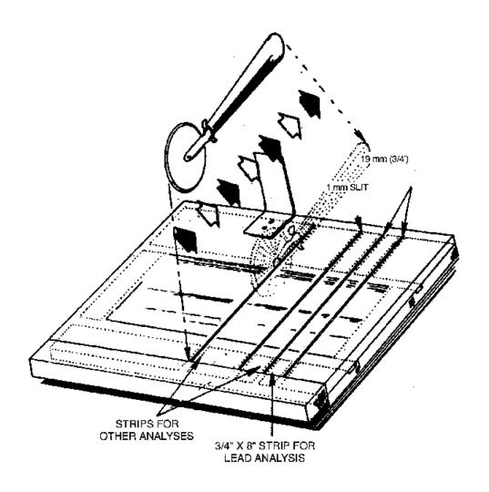
Figure 2. Diagram of filter cutting procedure.
