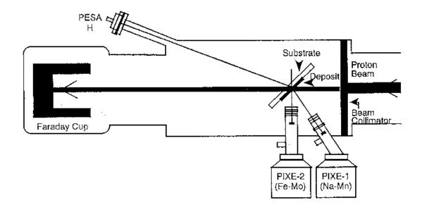
Figure 1. Example of schematic of a typical PIXE thin target system.
