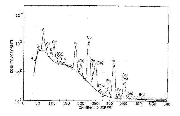
Figure 4. Example of spectrum for an indoor industrial aerosol.
