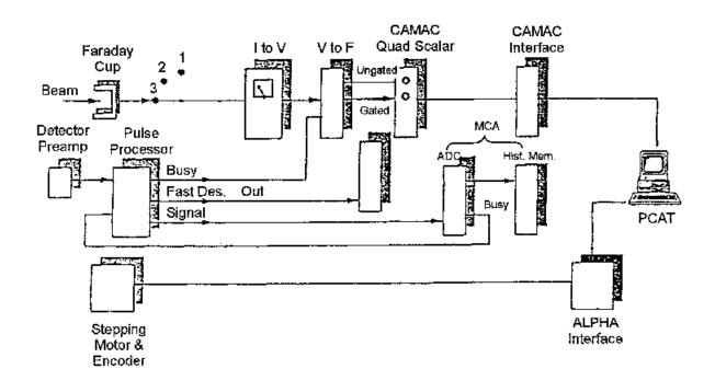
Figure 2. Example of PIXE Data Acquisition System.
