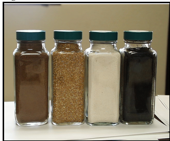
Figure 3: Arsenic Treatment Media
