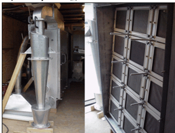
Cyclone sampler (left) and filter carriers (right) for collecting large amounts of PM.
