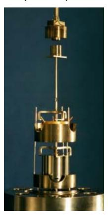
Sinkers and magnetic suspension coupling comprising the heart of the densimeter. The electromagnet at the top hangs from the balance and levitates the permanent magnet below it. In this photo, the bottom sinker is being weighed, while the top sinker sits on its rest. This assembly is normally contained within a pressure vessel.
