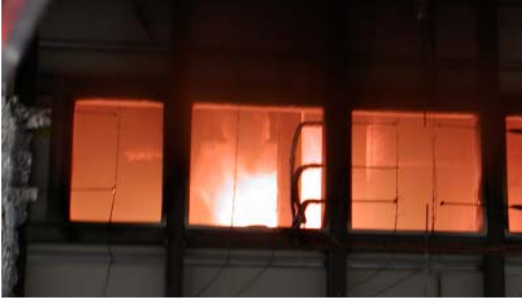
Figure 5. View of compartment from air exhaust outlet several minutes after the start of test 6. Note the flame impingement on the steel trusses and bar.
