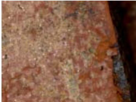
700 °C for an hour mud cracks partially obscured by formation of whiteish “sandy” phase on surface delamination easy with finger
