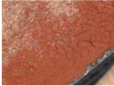
250 °C for an hour mud cracks much more visible
