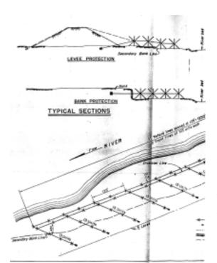
Fig. 8: How jetty jacks protect levees (top), banks (middle), and how the jetty field is configured for bank stabilization and levee protection (bottom). Source: U.S. Army Corps of Engineers 1953.
