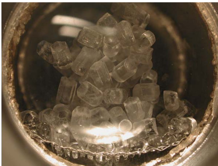
Fig. 3.5. Methane pellets in a collection vessel [3.3.2].
